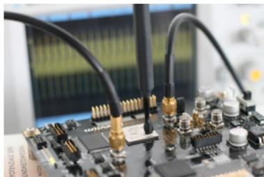
**Figure:** Power analysis setup.
